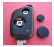
For TWO buttoned remote you would need to open it and separate all parts for inserting new buttons from inside.
