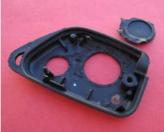
Old rubber buttons should be removed by pushing it through with the small screw driver. If any remnants of an old buttons are still left around holes they need to be scraped off/cut out with Stanley knife. Be careful not to damage plastic shell.
