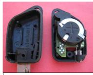
Once you open your remote you end up with bottom part ant top part consisting electronics and plastic button shell.
