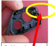
Rubber piece for holding LED light should be left intact.
