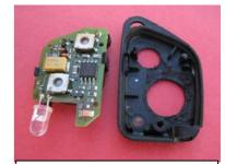
You should end up with clean top plastic shell and electronic board with switches free of plastic tips, ready for inserting buttons, as shown above.
