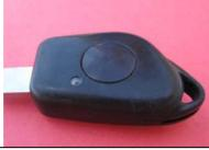
For **ONE buttoned remote** simply remove any remnants of the old rubber key button from outside of remote (no need to open remote) and press fit new Silicone button in. Your remote will work without any need for programming.
