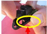
Carefully lift electronics up, not to damage plastic supporting pins from the top part of remote.
