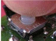
Next remove deteriorating plastic knobs from the top of switches. Simply scrape them off using your finger nail.
